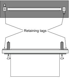
4. Fasten the two retaining screws clockwise and the retaining tags will expand until the base is securely installed.
