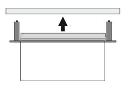
3. Push upwards the base. Make sure that the retaining tags are not expanded.
