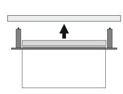
3. Push upwards the base. Make sure that the retaining tags are not expanded.
